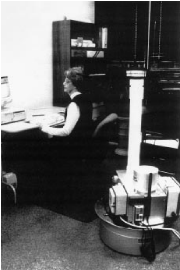
Figure 1 The portable air sampling device (PASD).
